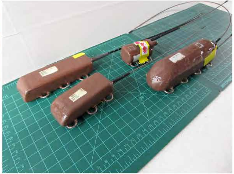
Figure 18. View of conventional VHF radios (foreground) and GPS logger radios (back), used for gharial tracking, and designed and built by ATS (Advanced Telemetry Systems, Isanti, Minnesota USA). The life of these units is 2-3 years, have a range of 1-4 km, and weigh 100-300 gms. A temperature circuit can be integrated to allow ambient readings of unit.
